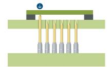
Use an extended stroke ESD ground probe to contact a ground point on the UUT to bleed off static before other probes contact a board.
