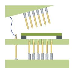
4. Use an extended stroke probe when connecting to transfer points that are connected to topside probes or other signals for sensor plates used in an upper gate assembly. This allows electrical verification to be performed while the topside assembly is in the "open" position.
