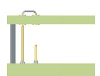
Used with a shorter stroke probe, the extended reach probe contacts a conductive sensor on a gate or support plate to signal if a gate is open or closed.
